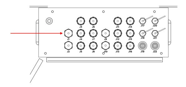
2. Attach a blue trunk TEE to the first trunk line, set digital voltmeter to "Ohms ( $\Omega$ )"; check and document the following pin-to-pin resistances (see worksheet below), repeat for all other trunk lines.
