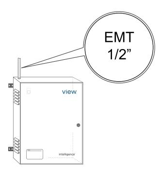
10. Furnish Line, Neutral, and ground wiring from the upstream panelboard to the CP. Typically this should be 12AWG THHN wire per NEC table 310.15(B).
