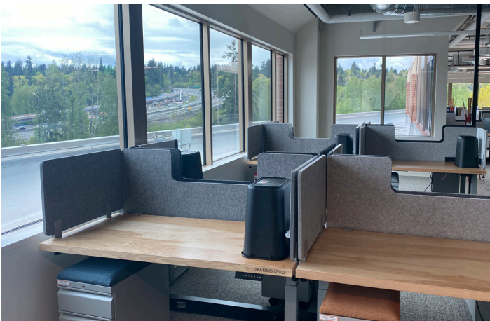
With desks perpendicular to the windows, the sun does not cause reflected glare on computer screens or direct glare into the occupants' eyes 2
