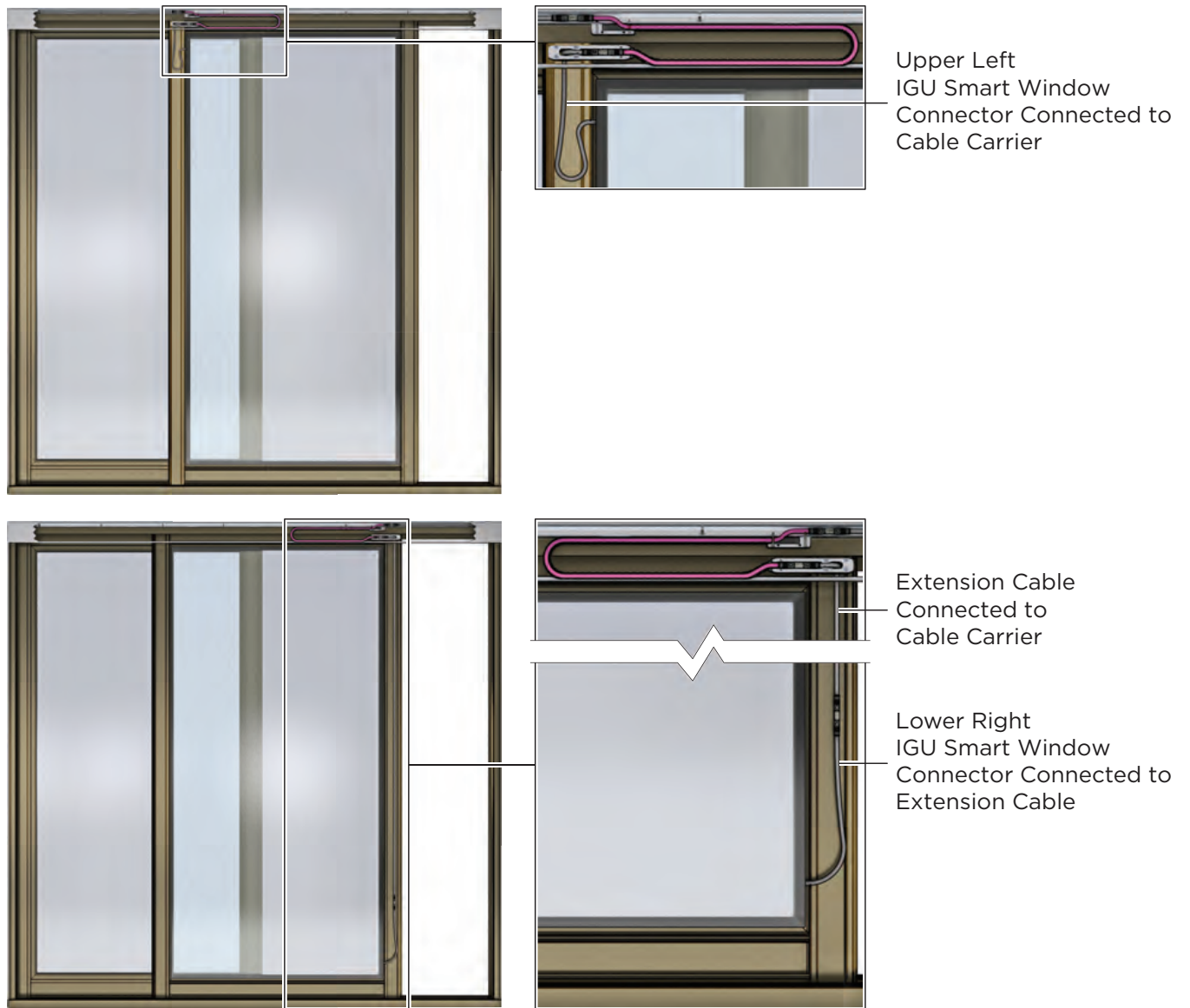
Cutaway views of OX sliding doors showing IGU Smart Window Connector connections in left and right stiles of door.
